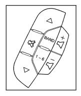
If your vehicle has this feature, some audio controls can be adjusted at the steering wheel. They include the following:
